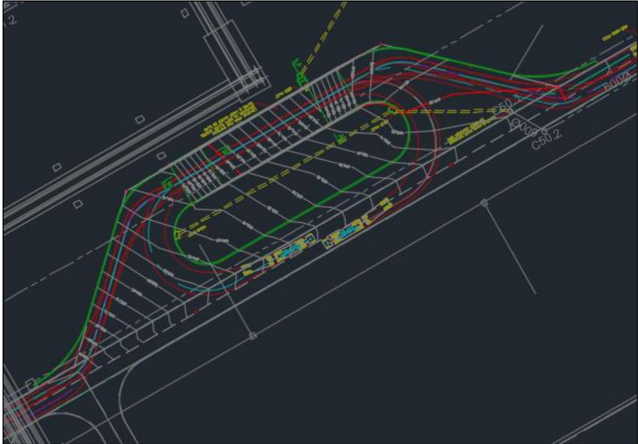
Figure 20: Gypsum loading platform contour detail
